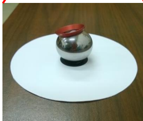
Illustration showing how the SMR sits on the fiducial target.
